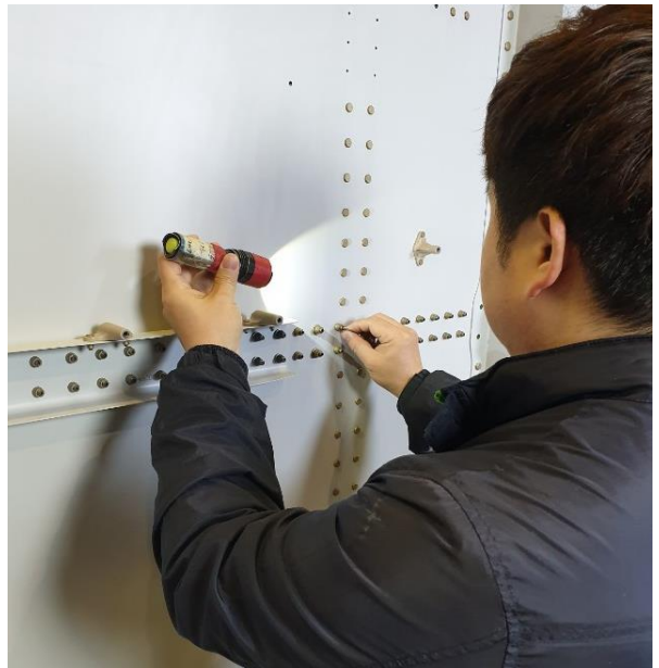
787 AWWB HI-LOK BOLT INSPECTION
